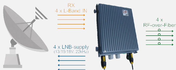
Functional Diagram 4 x optical TX (transmitters)
