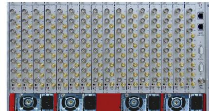
The “**FlexLink K7 Pro**” features variable gain-control & slope-equalization, RF power monitoring as well as a 10MHz reference signal port. Furthermore, it supports status monitoring of all active components and comes with 1:1 redundant dual power-supply (hot swappable). Additional flexibility is being provided via available options like switchable LNB-supply, individually selectable and configurable for each input.
